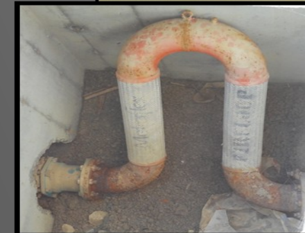
Severe Corrosion of Buried Firewater Line
