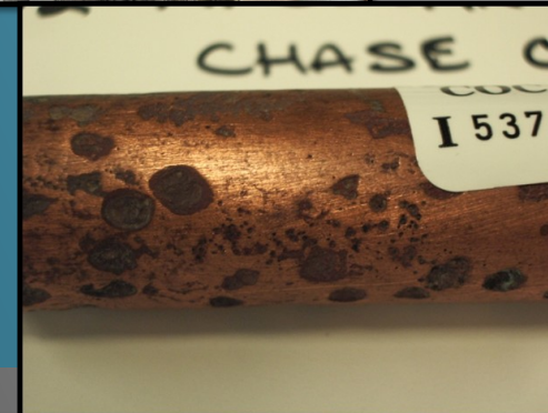
Severe Pitting Corrosion on Buried Copper Water Lines
