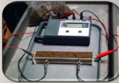
soil box resistivity test
